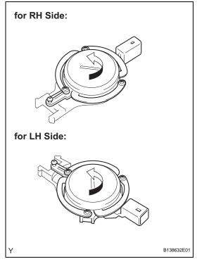
(c) Remove the roof speaker by turning it in the direction of the arrow shown in the illustration.
